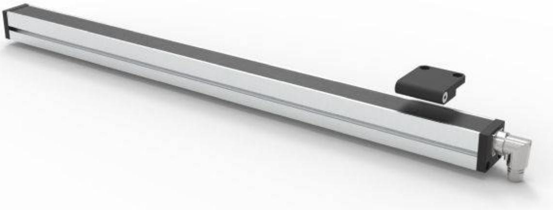
The mounting distance between the reference magnet and the detecting region is not critical, from 5 to 20mm. The encoder is tunable and programmable using PC software.
