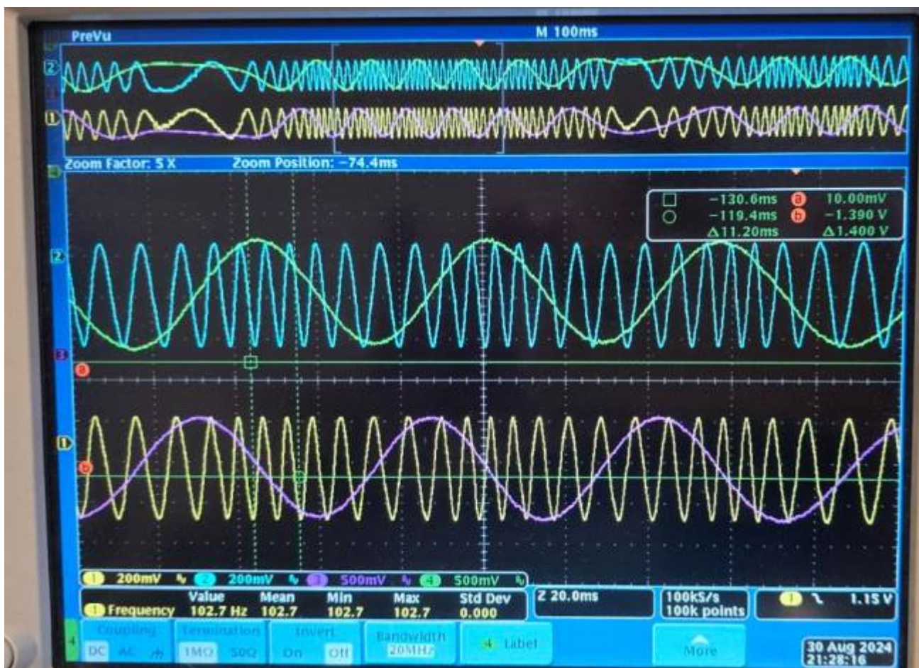
Example of SIN/COS Output (Blue and Yellow) with the encoder configured with 2mm of sine period.
