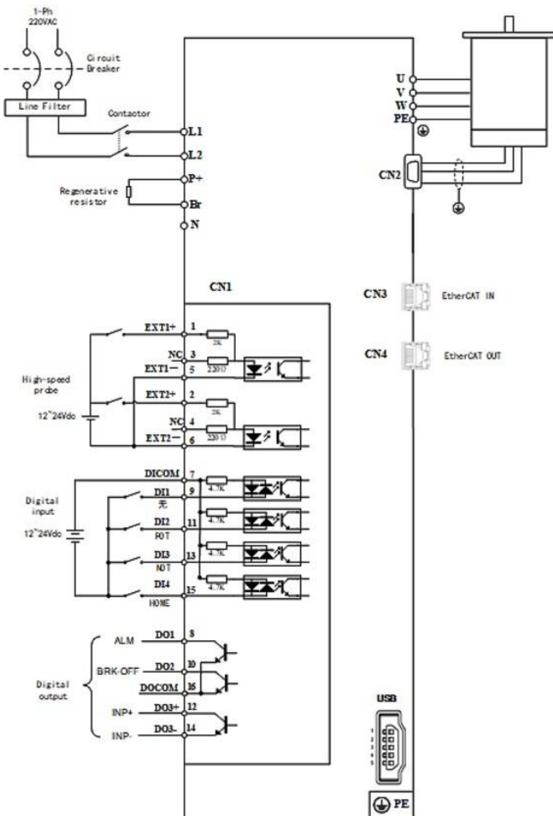
NL7-RS series servo drive supports single phase and three phase 220VAC. Only driver with power rating above 1500W supports three phase 220VAC.
