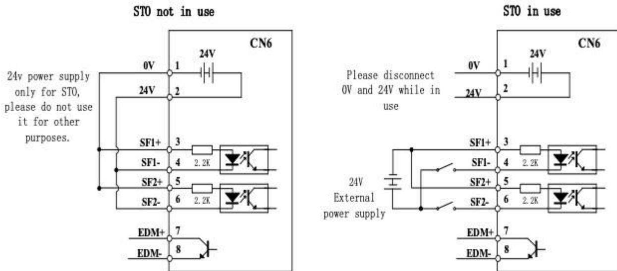
Please take precautions when enabling STO functions as servo drive will lose control over the motion of the motor. Motor might dropped under gravitational pull (vertically mounted load) or moved when external forces are re applied to it. Alternatively, motor with holding brake can be chosen.
