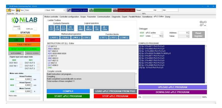
The IL compiler check for sintax and logical error and then compiled the program for the internal PLC. After the building phase the user must download the program into the motor using the DONWLOAD button.
