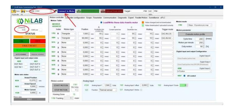
3. Please verify that the expert window is disable and tghe write encoder / commutation parameters in the motor option is unchecked.
