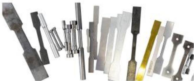
Metals are widely used in the automotive and construction industries. Key measurements for metals include r-value, n-value, modulus, tensile strength, strain, offset yield, and upper and lower yield strength. Common metals testing standards include ASTM E8, ASTM A370, and ISO 6892.
