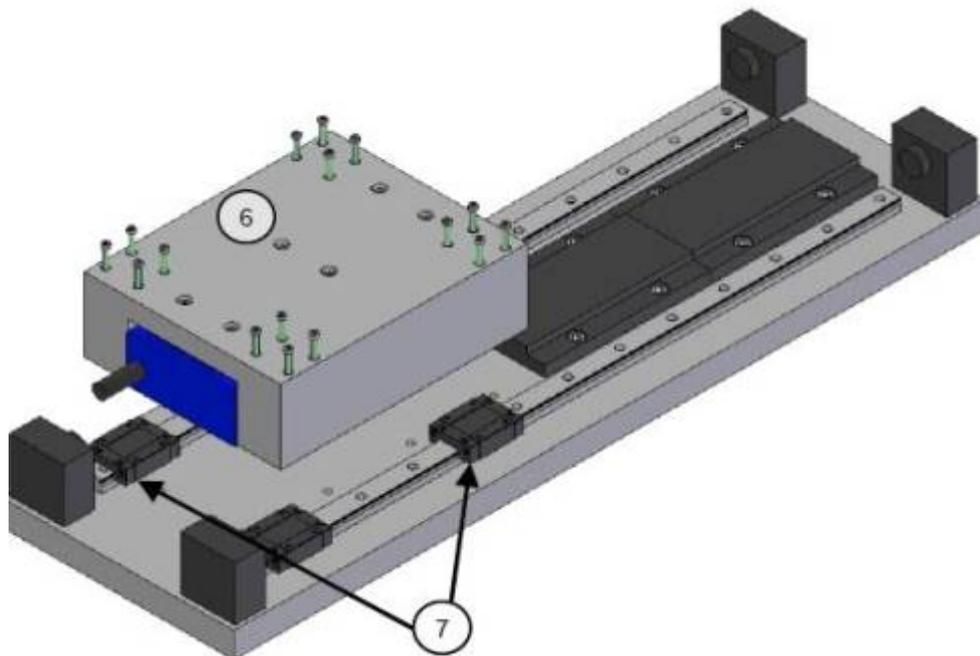
4: Slide the motor assembly (8) over the mounted magnetic ways and temporarily secure the motor against the mechanical end stop.
