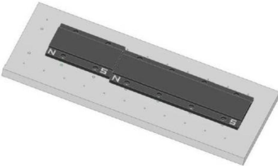
Then the primary part will be set up with the cables coming out towards the north pole of the secondary part. Otherwise, the motor phase sequence U, V, W will not be preserved.
