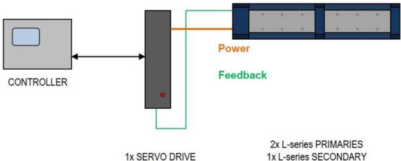
In a parallel arrangement the primaries in feed direction can mechanically be coupled and be arranged in succession. To ensure successful operation, the primaries must be arranged in a specific grid. The determination of the grid sizes that must be adhered to depends on the direction of the cable entry and the permissible bending radius of the power cable.
