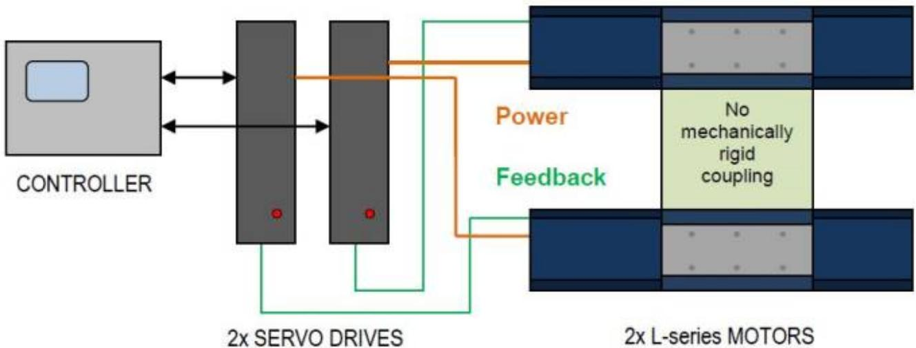
With gantry arrangements the motors may be stressed asymmetrically, although the position offset is minimized. As a consequence, this permanently existing bias load may lead to a generally higher stress than in a single arrangement. This must be taken into account when the drive is selected.
