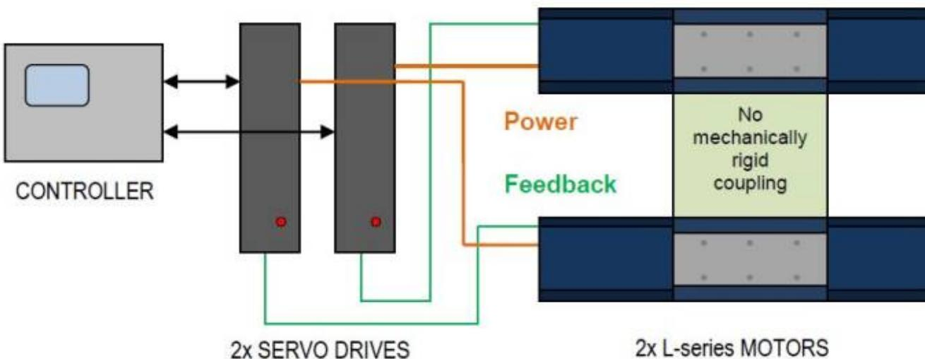
With gantry arrangements the motors may be stressed asymmetrically, although the position offset is minimized. As a consequence, this permanently existing bas load may lead to a generally higher stress than in a single arrangement. This must be taken into account when the drive is selected.
