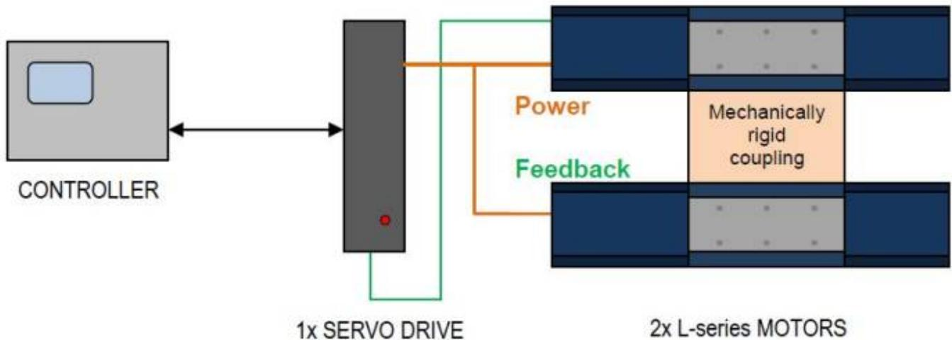
To ensure successful operation, the axis must fulfill the following requirements in parallel arrangement:
