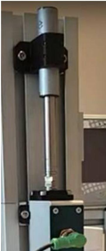
In vertical applications, when the roto-linear motor is not powered, the linear axis can fall down due to gravity. Using MagLift, the gravitational force is counterbalanced and the linear motor remains in steady state. 6 force sizes are available : 12, 17, 22, 40, 50 and 60 N, respectively MagLift12, MagLift17, MagLift22, MagLift40, MagLift50 and MagLift60.
