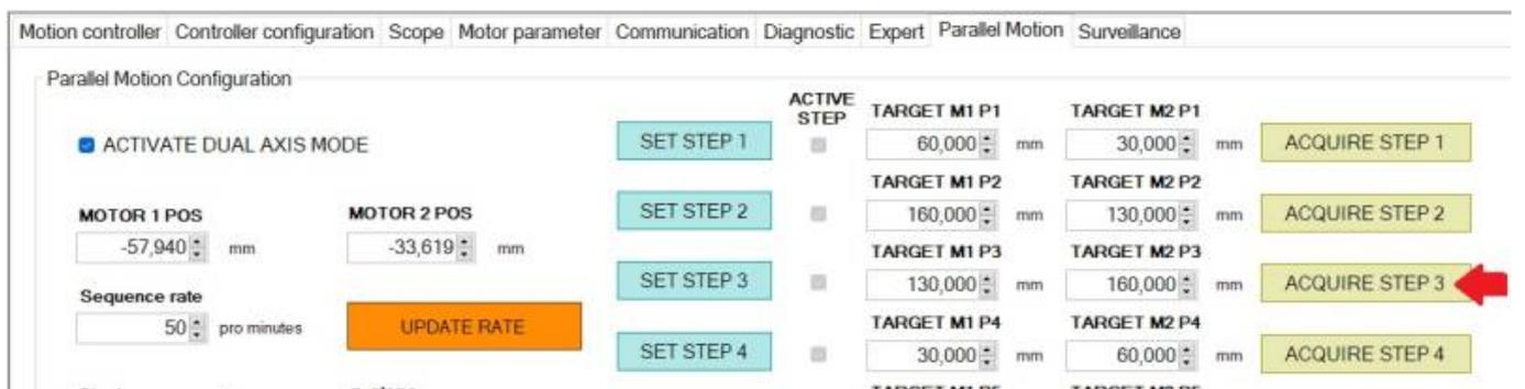
Move the robot in the starting position and store the fourth positions using ACQUIRE STEP 4 button.
