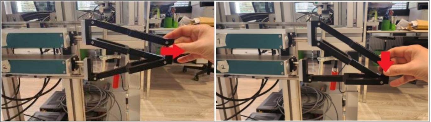
Press button Acquire Step to capture the position of the two axis. If the number are with digits you can correct using the number field and press the SET STEP 1 to store.
