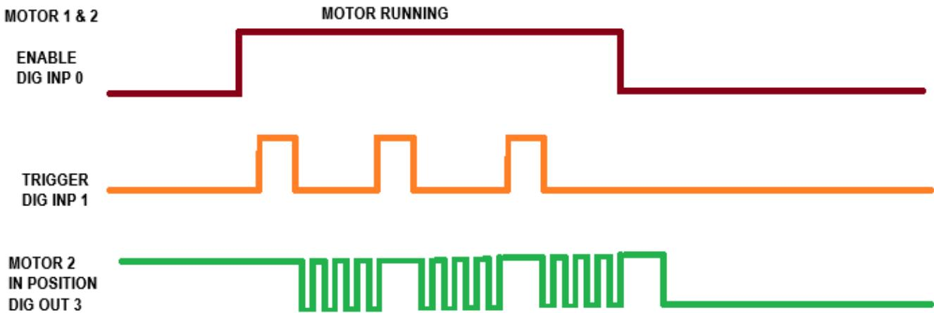
At every Disable, Digital Input 0 low the two motors executes Automatic Homing to reach the parking position.
