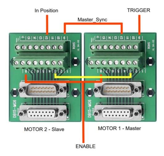
The signal must be connected together as in the table below (with reference to the photo above)
