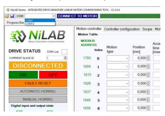
Then, you have to select the right one on the combobox list in the NiLAB Starter Software and then press the button "Connect to Motor".
