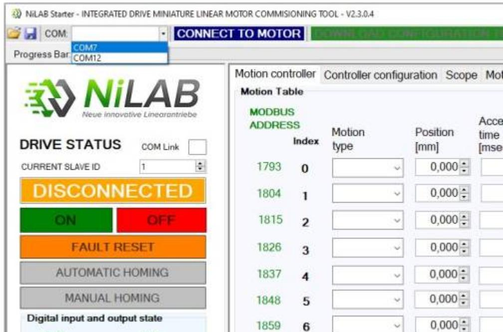
Then, you have to select the right one on the combobox list in the NiLAB Starter Software and then press the button "Connect to Motor".
