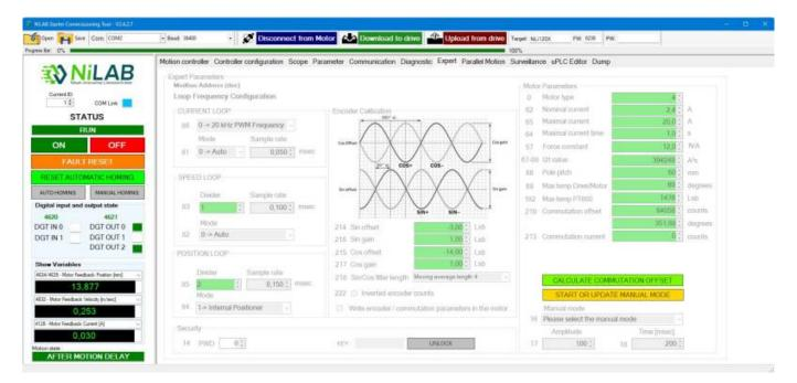
**Servo drive optimization:** the optimization procedure inside the controller/driver (control loop tuning) is possible using the controller configuration window inside NiLAB Starter Windows Software (Link: NiLAB Starter).
