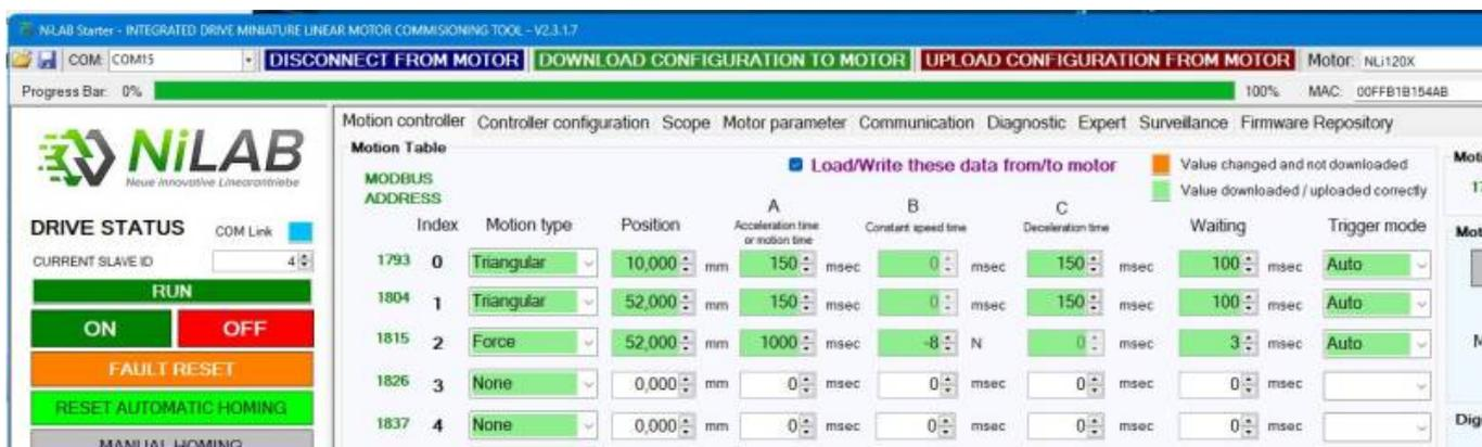
The sign of the force specified in the table must correspond to the direction of the slider, as in this photo.
