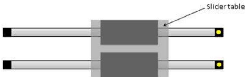
Both forcers must be oriented in the same direction on their shafts. It is suggested that the end of the forcer that has the serial number be pointing toward the end of the shaft that is marked with yellow paint. If the orientation of the coils is different, it is possible to have a totally inoperable or a runaway system, or it will cause significant loss of thrust. The standard for parallel drive system is mirrored cable exit locations. See drawing below.
