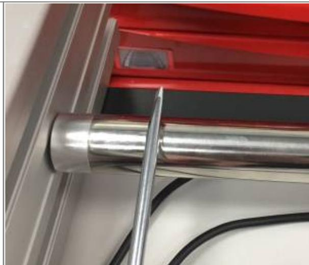
Position when the magnets start. (close to the shaft end)
