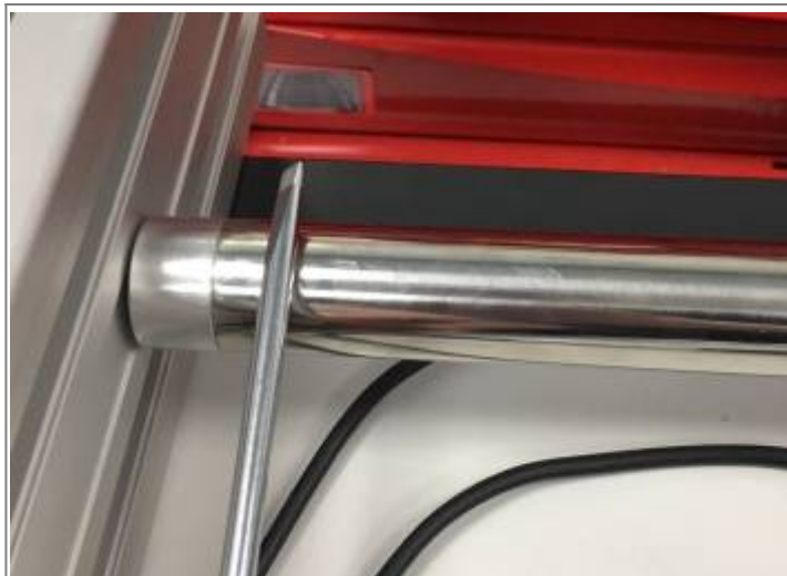
Position when the magnets start. (close to the shaft end) Yellow point is on this side
