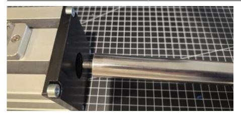
Mount again the end stop on the internal screw of the slider
