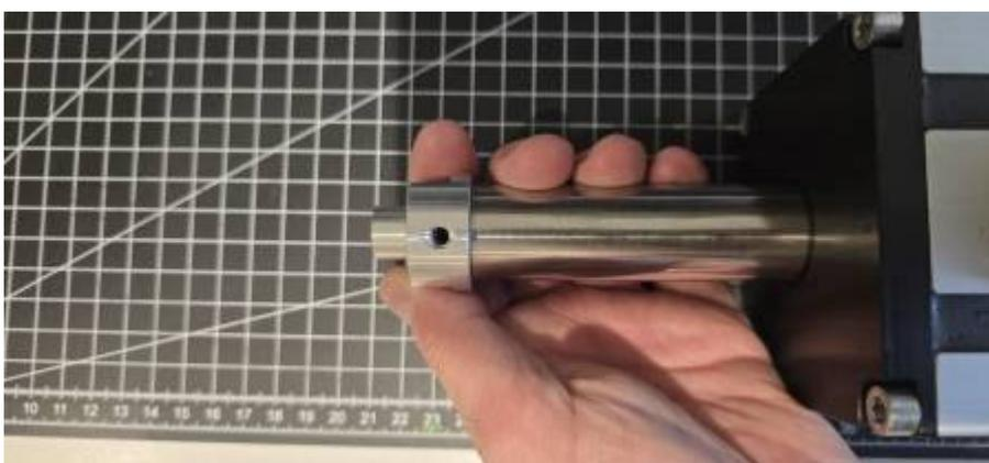
Screw the grub screws to avoid the end cap rotation.
