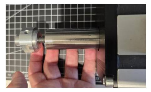
Close completely the end cap reaching the stainless steel rod end.
