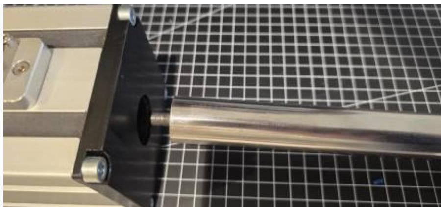
Mount again the end stop on the internal screw of the slider
