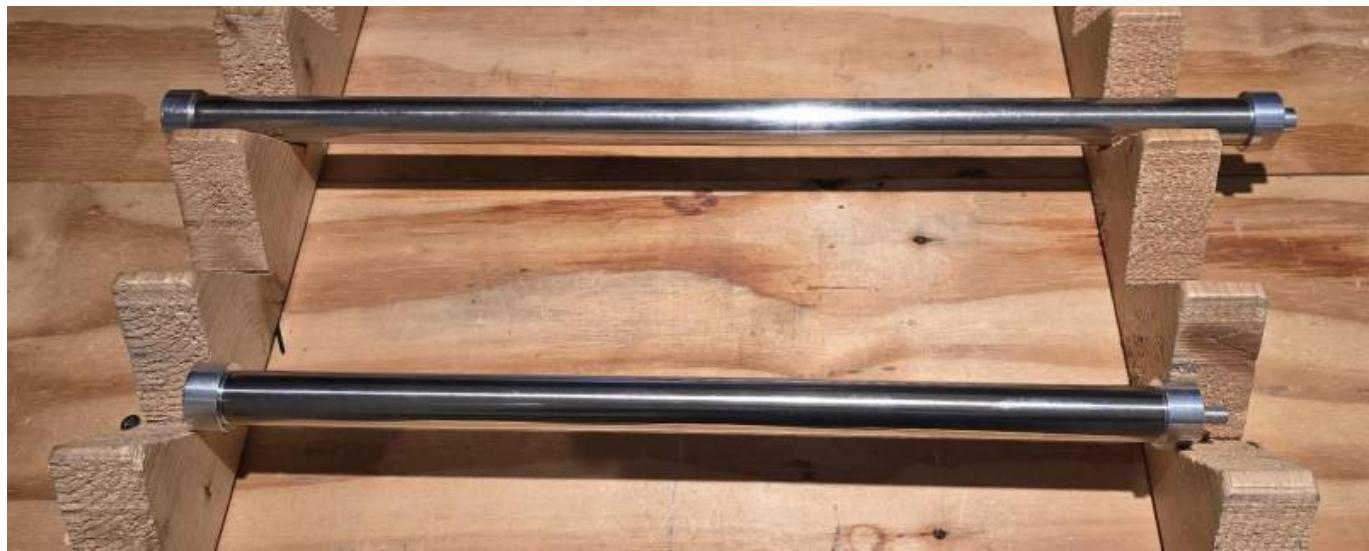
**To decouple the two rods joined by attraction force, first rotate one slider by 90 degrees to reduce the force, and then complete the decoupling by applying the necessary separation force.**
