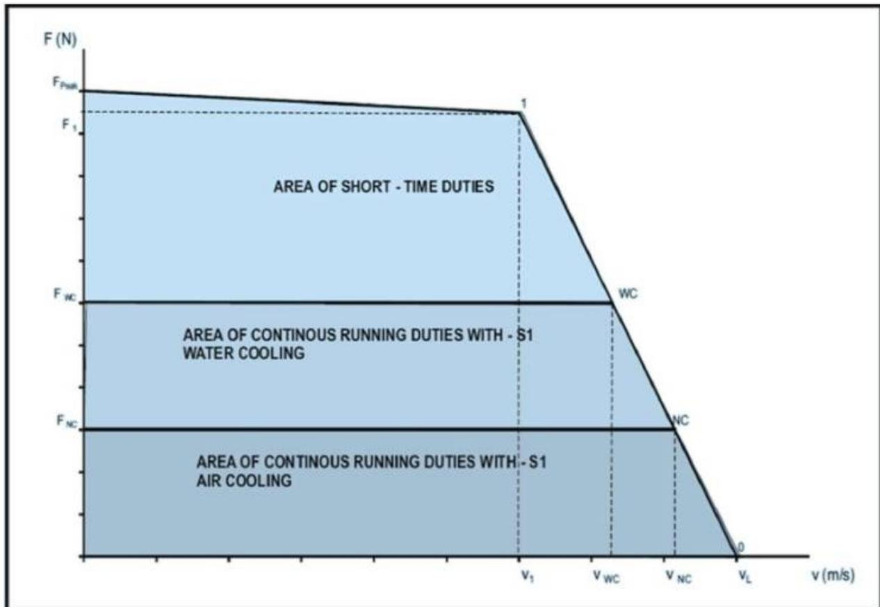
When the velocity rises, the available DC bus voltage is reduced by the Back EMF of the motor. This leads to a reduction of the maximum feed force at higher velocities. The characteristic curves are specified up to the continuous nominal force. The velocity that belongs to the continuous nominal force is known as nominal velocity,  $v_{NC}$ .
