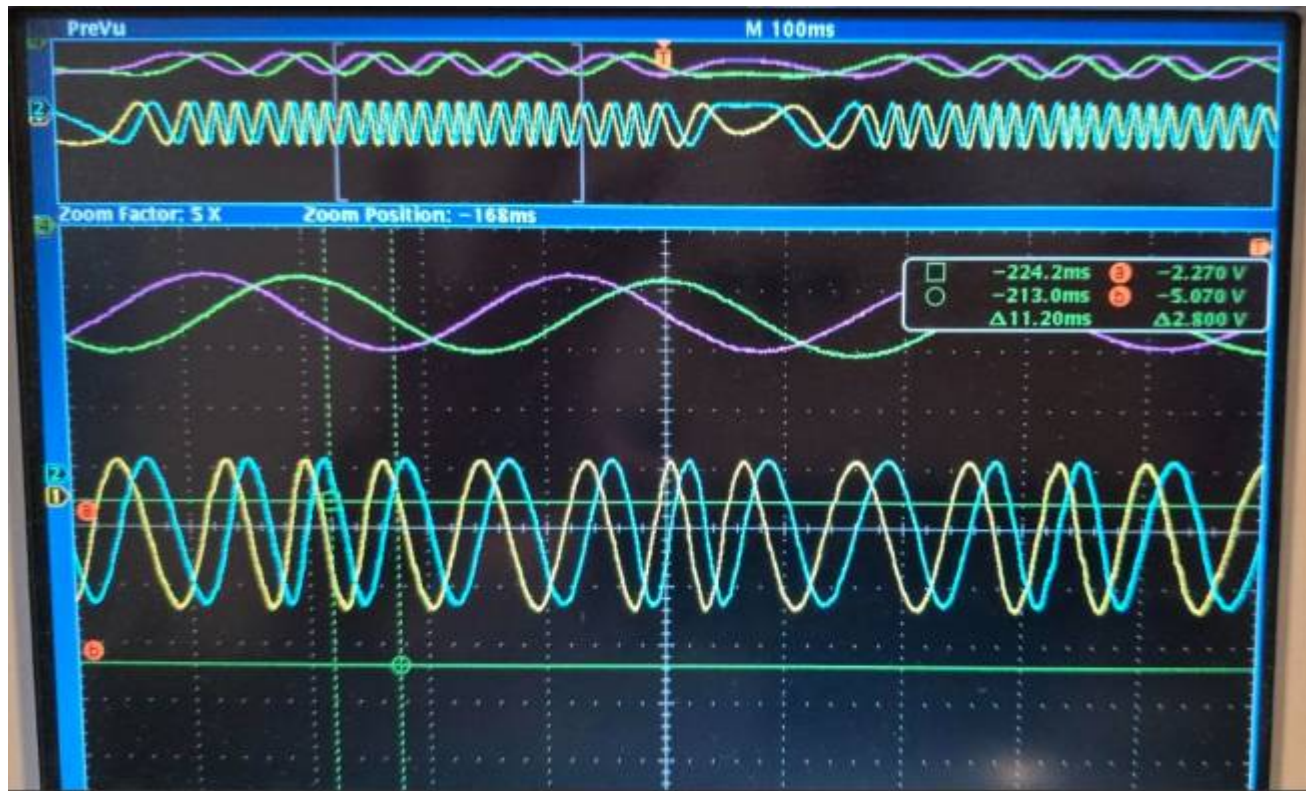
Example of SIN/COS Output (Blue and Yellow) with the encoder configured with 4mm of sine period. The signal in green and violet are the signal (with 32 mm of period) detected by the internal analog sensor before the conversion and conditioning.
